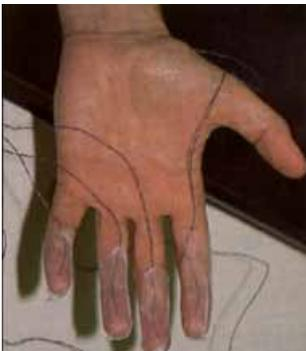
Hand fitted with thermocouples
