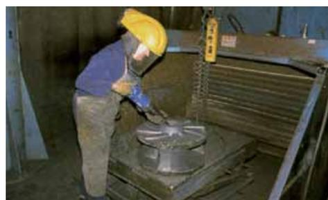
Low-vibration chipping hammer knocking out a casting
